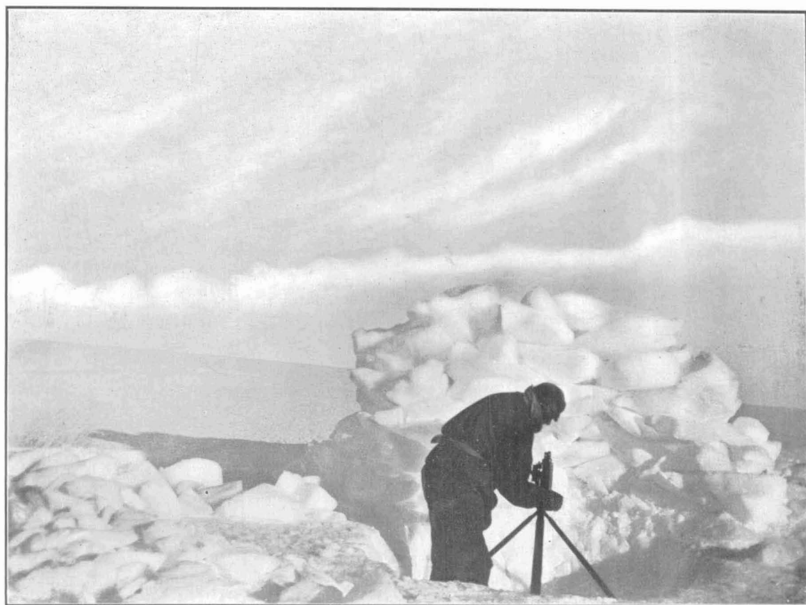
Fig. 2.—Station 1E. E. N. Webb Observing with Dip-circle in a Pit-and-Screen Shelter in the Glacier Ice of the Plateau Slopes.
