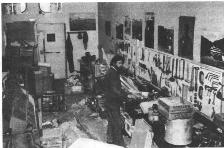
Plate 6. The plumbers' workshop including tools, a metal press, guillotine and oxy-acetylene welding gear. (Antarctic Division photograph by P. Sullivan)
