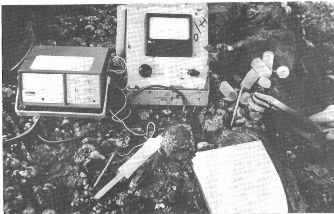
Plate 10. The portable hygrometer (left), thermistor thermometer (centre) and their sensors (foreground) which were used to measure the relative humidity and temperature of substrate.
