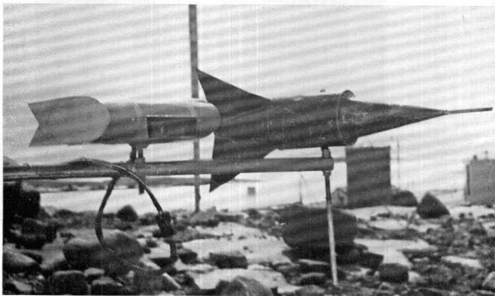
PLATE 1. PE gauge and Mellor rocket trap set at the one level for calibration.
