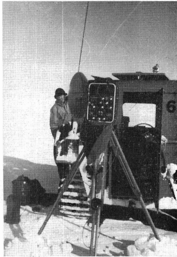
PLATE 4. Tellurometer with 17-inch circular reflector. The muff-cover around the instrument reduced heat losses from crystal oven.
