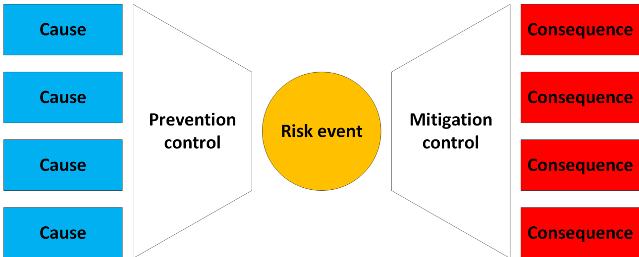
Figure 5.1. Bowtie model of risk analysis. On the left of an identified event are the hazards and preventative measures, on the right of the event are the recovery measures and consequences.
