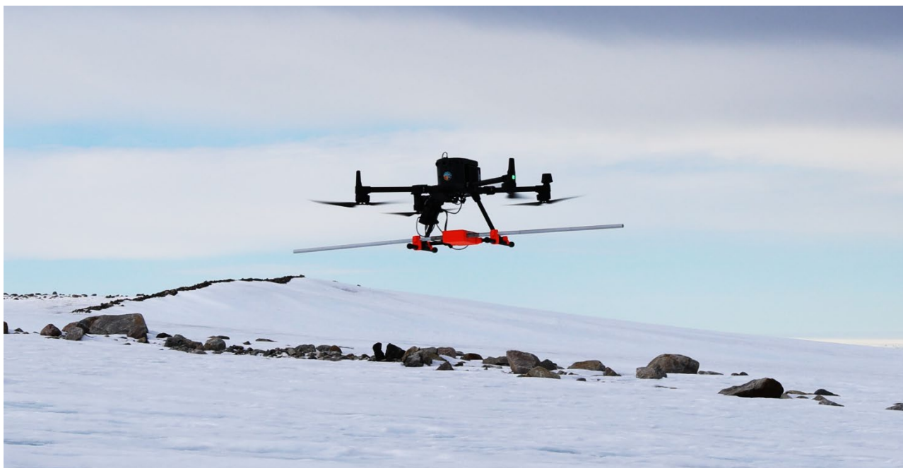
DJI M350 with Ice Penetrating Radar payload at Loken Moraine, near Casey Station (photo Gwil Price).
