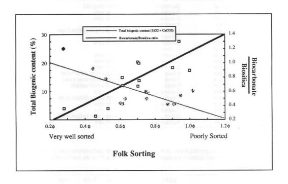
Figure 8. Plot of total biogenic content as a percentage of whole sediment and biogenic carbonate/biogenic silica ratio against folk sorting for samples to landwards of the shelf break. This plot demonstrates that the total biogenic component is highest in areas that are subject to the most reworking. Further, a loose association between sorting and the biogenic carbonate/biogenic silica ratio indicates that higher energy areas prevent the deposition of diatom frustules.
