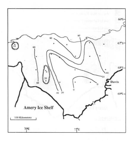
Figure 7. Contour plot of sand proportion in Prydz Bay. Sand percentages are highest in the north of the Bay where the finer fractions are removed or are prevented from settling out. Very low values in the vicinity of the Amery Ice Shelf indicate an area not being reworked. The low value in the northwest is the result of the very high proportion of biogenic material in that sample.
