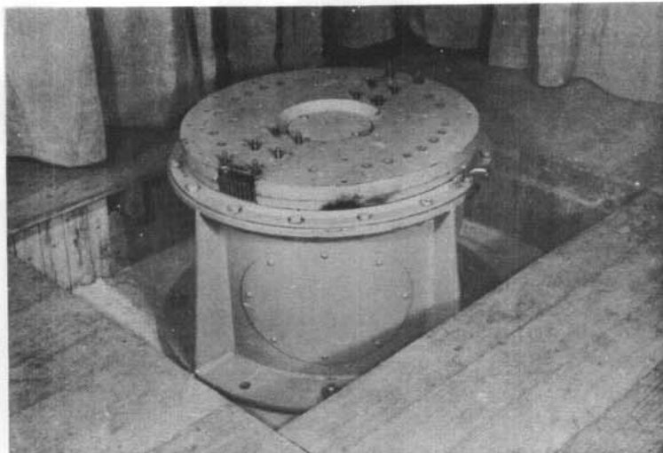
FIG. 2. BASE AND TURNTABLE OF TELESCOPE.
