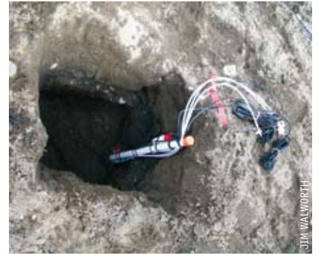
This mini-piezometer, with an oxygen sensor attached, is used to take water samples to measure groundwater chemistry.
