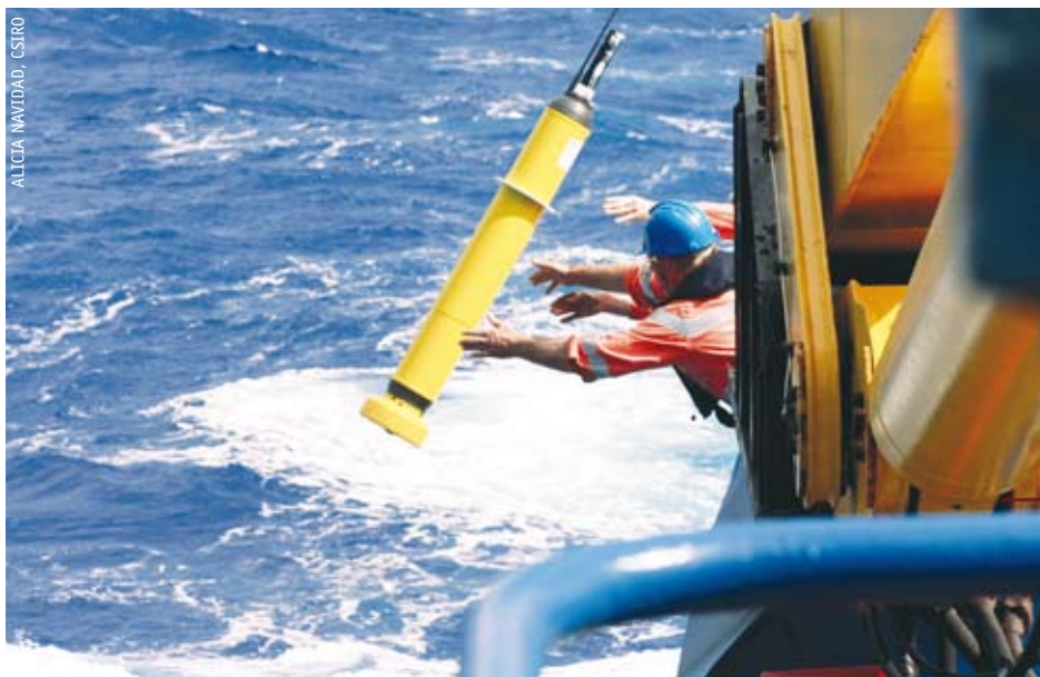
One of 30 Argo floats is deployed in the Australian sector of the Southern Ocean during the International Polar Year. The floats join a network of 3000 around the globe measuring temperature and salinity in the upper 2000 m of the world's oceans.
