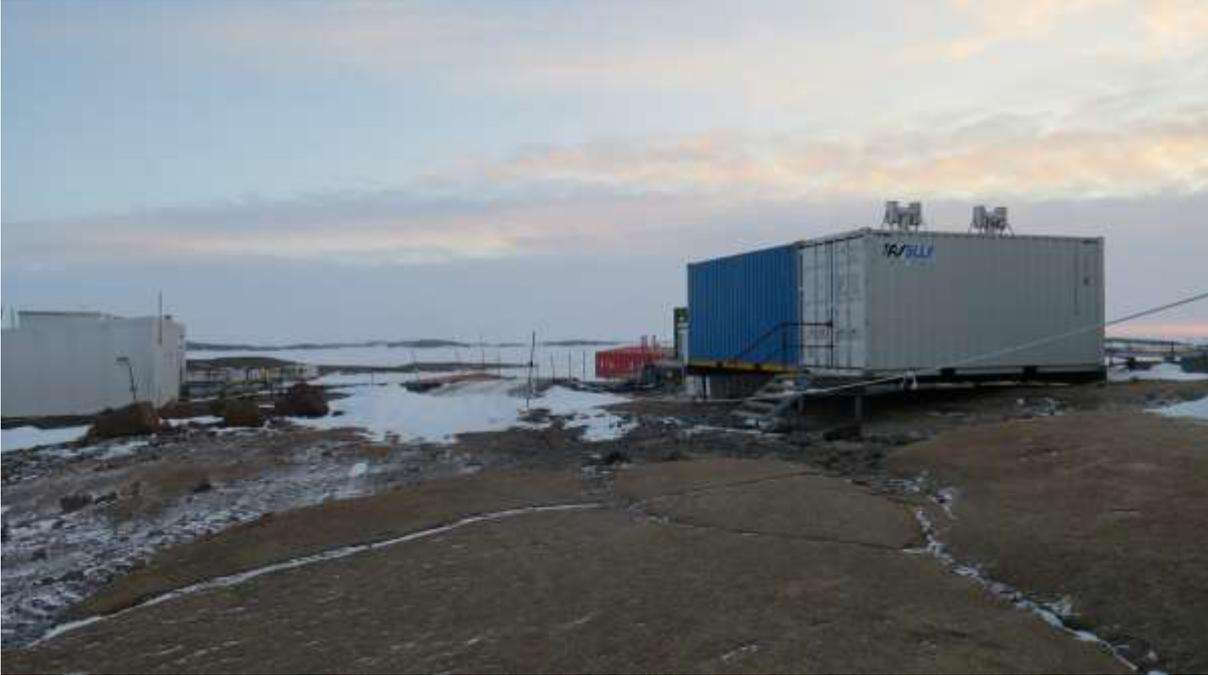
White container is entry/cold porch and blue containers are wet and clean lab spaces. The space between the two lab containers will have shelving and storage. Entire interior will be insulated.
