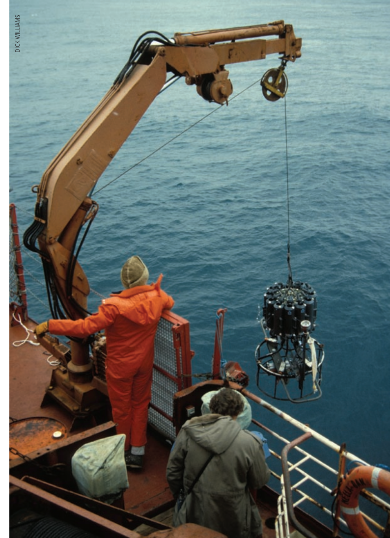
Above: ‘CTD’ probes, measuring Conductivity (salinity), Temperature and Depth, are lowered from the helideck during a 1986–87 marine science cruise.
