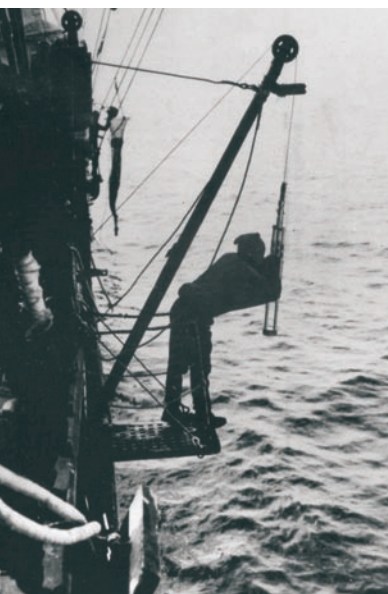
Alf's skills as a gymnast stood him in good stead to balance on the Discovery's outboard platform, making oceanographic measurements with his Nansen-Pettersen waterbottles.
