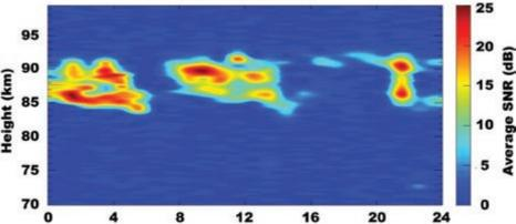
Polar Mesosphere Summer Echoes (charged ice aerosols) detected by radar over Davis on New Year's Eve 2007 (SNR = signal-to-noise ratio; dB = decibels).
