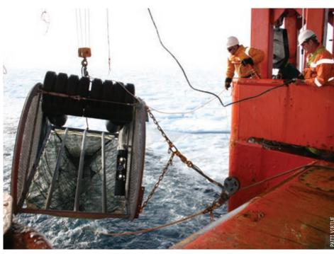
The Surface and Under Ice Trawl, being deployed from the Aurora Australis, is equipped with a high-resolution video system to film the subsurface of the sea ice.
