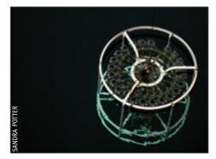
Deployment of Conductivity, Temperature and Depth (CTD) sampling bottles.
