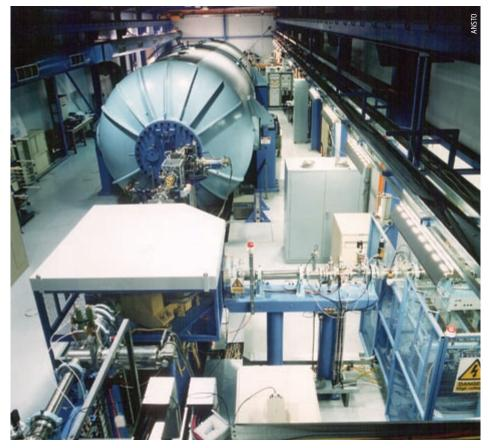
The 10 million volt particle accelerator – the Australian National Tandem Accelerator for Applied Research – at ANSTO is used to measure beryllium-10 signatures in ice cores.
