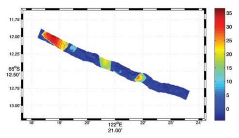
Figure 2: Sample of an approximately 2 km flight track of laser scanner-derived surface elevation [m] over the Dalton Iceberg Tongue showing some bigger icebergs enclosed by sea ice.
