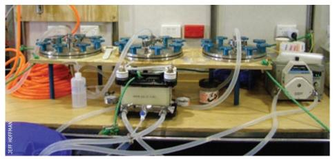
Water samples collected in the Southern Ocean were passed through three filters (stainless steel racks pictured) of decreasing pore size – 3, 0.8 and 0.1  $\mu$ m – to separate phytoplankton, zooplankton, microbes and viruses. The outflow from the 0.1  $\mu$ m filter was collected and further concentrated in the 'tangential flow filter' at the front. The 0.1-0.8  $\mu$ m fractions, which contain the majority of archaea and bacteria, will be sequenced.
