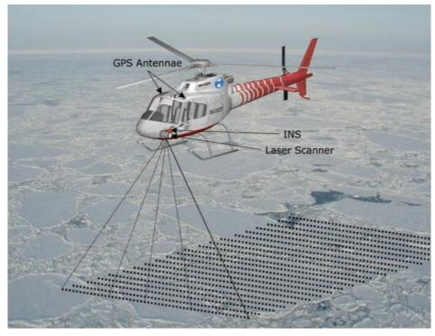
Figure 1: The laser scanning principle.
