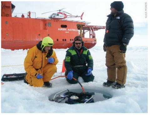
Marine Science Support members Alan Poole (left), Peter Raymond and Andrew Cawthorne, deploy an instrumented Remotely Operated Vehicle through a drill-hole beside the ship during SIPEX.
