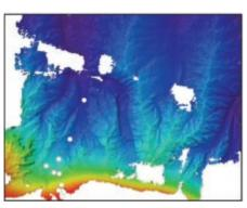
A 90km-wide plan-view of the 3-D seascape in the CEAMARC study area. The circles are sample sites targeting the deep and rugged submarine canyons draining the George V shelf. White patches indicate areas where multibeam data is missing. The shallower continental shelf is coloured red to yellow.
