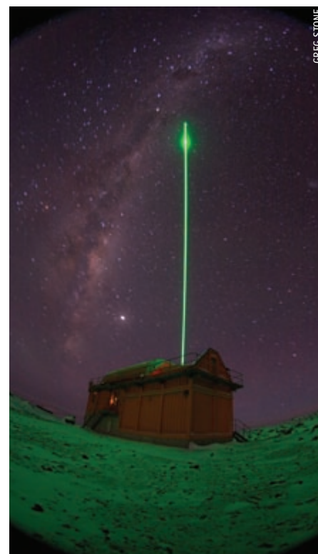
The Davis lidar uses pulsed light from a powerful laser to map polar stratospheric clouds and measure atmospheric temperatures.
