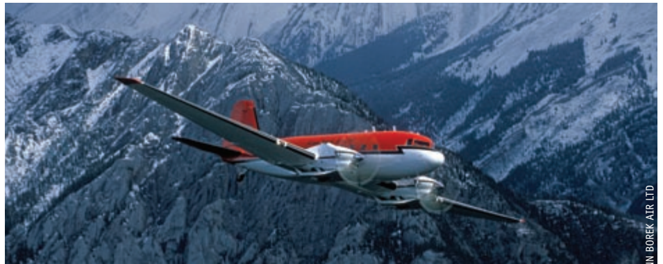
A ski-equipped Basler BT-67 turboprop (an upgraded DC-3) from Kenn Borek Air Ltd, of Canada, will carry a suite of geophysical instruments to explore the glaciological and geological properties of the vast Aurora and Wilkes subglacial basins.
