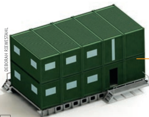
Drafter's impression of the Wilkins Runway living quarters, mounted on a sled. The structure contains the mess, kitchen, lounge, laundry, shower and toilet facilities, a plant room and a multi-purpose room for computers, gym and emergency accommodation.
