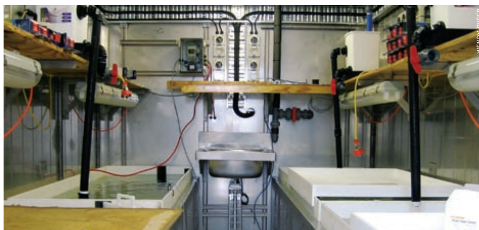
Inside the shipping container are four seawater tanks, and small heaters on the shelves above, which regulate the temperature of the water depending on the experiments being conducted. Other experimental equipment can be installed on the shelves as required.
