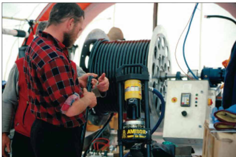
The hose reel and motor controller of the AMISOR hot water drill showing crimping tool for hose fittings.
