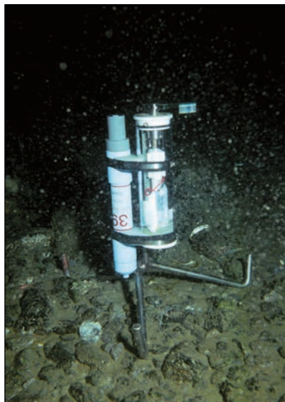
Light meter on the seabed near Casey, 15 m below the surface, which has been recording data for the last two years
