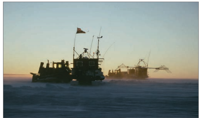
High on the Antarctic plateau, ice radar equipment is used to measure the thickness of the ice sheet
