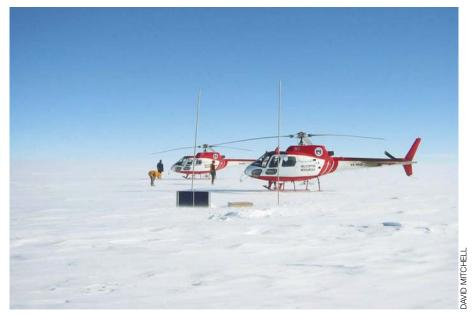
Deployment of Narod fluxgate magnetometer (housed in the box in the foreground)
