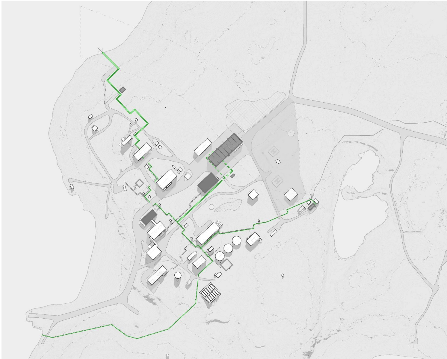
Figure 14. Proposed service reticulation pathway (green) within the DCIW proposed site plan for Davis station
