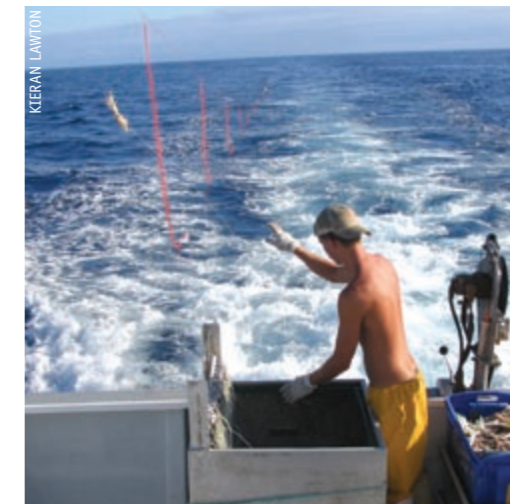
Lines were set using different bait types – in this case squid – to assess its effects on hook sink rate. Experiments were also conducted in conjunction with bird scaring lines (red streamers pictured).
