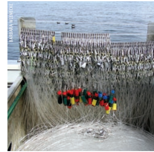
Sink rate recorders were attached to hooks to assess the effect of different lead weight characteristics, bait types and other factors on hook sinking.
