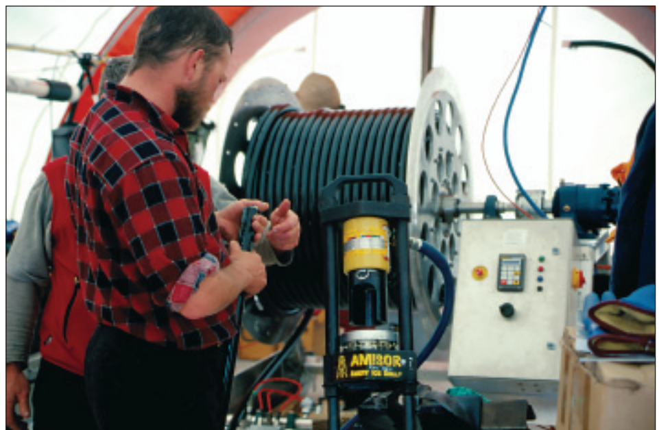
The hose reel and motor controller of the AMISOR hot water drill showing crimping tool for hose fittings.
