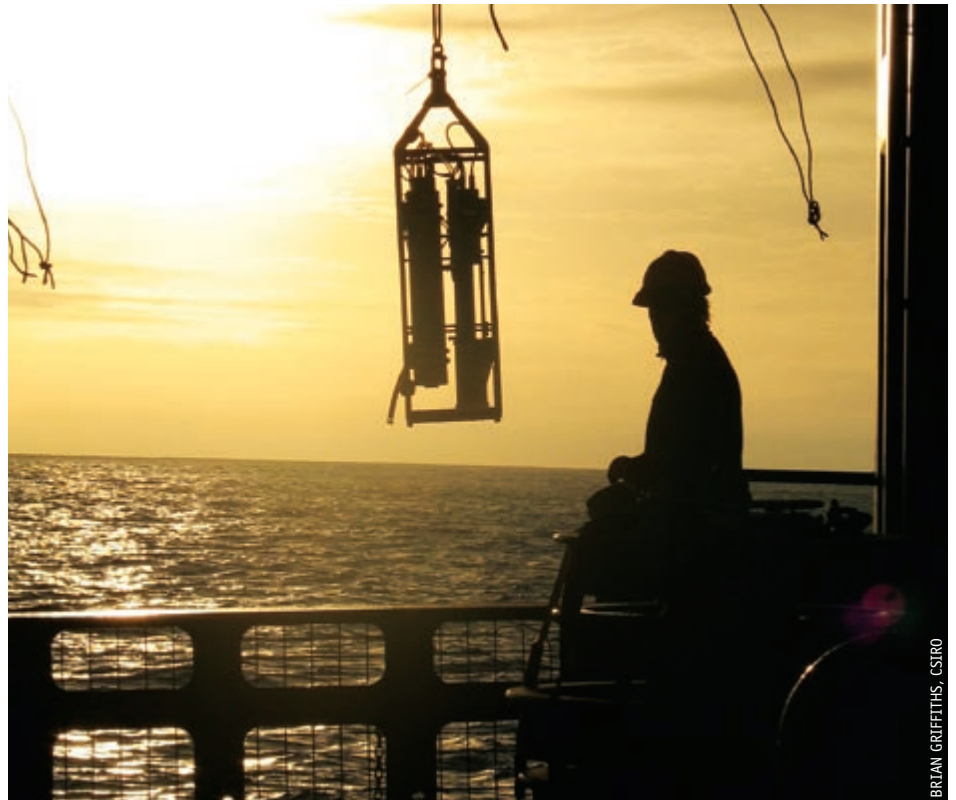
A WetLabs ac-s underwater spectrophotometer being deployed from the deck of the Aurora Australis.
