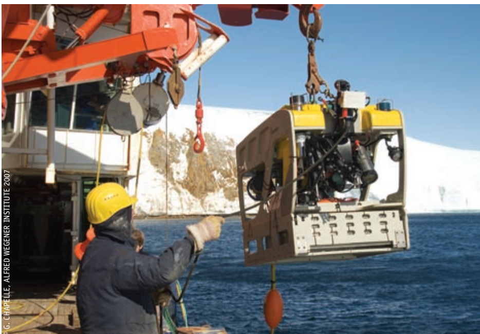
The Remote Operating Vehicle was used to capture still images and video footage, and collect some samples, during the voyage.
