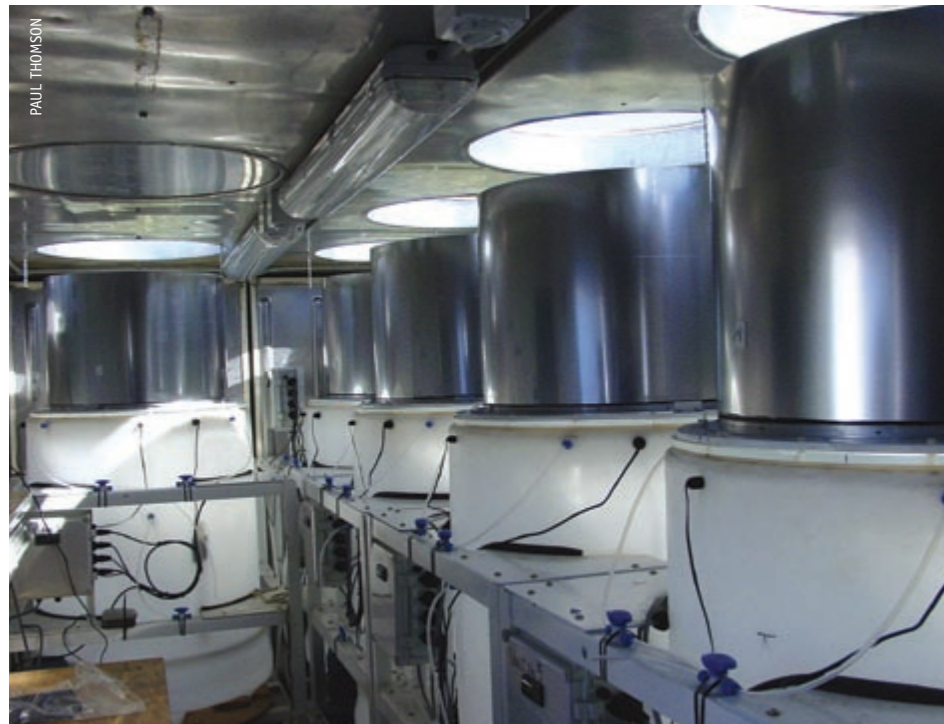
Marine protists were incubated for 13 or 14 days in these 650 L tanks. Reflective tubes conducted sunlight from the domes in the container roof. Screens on the top of each tank removed different amounts of UV radiation from the sunlight.
