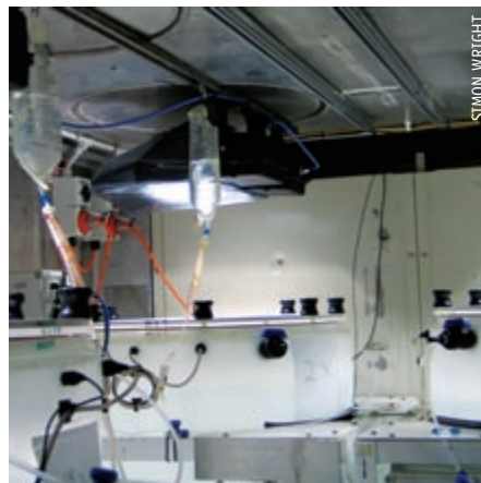
The 650 L gas-tight minicosm tanks use intravenous feeding bags (courtesy of the Polar Medicine Unit) to deliver acid slowly to each tank. Tanks have temperature control, gentle stirring, filtered artificial light, and several sampling points.
