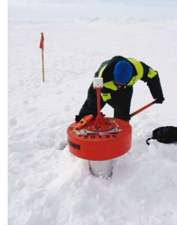
Anthony Worby deploys a buoy on a sea ice floe to gather information about sea ice drift.
