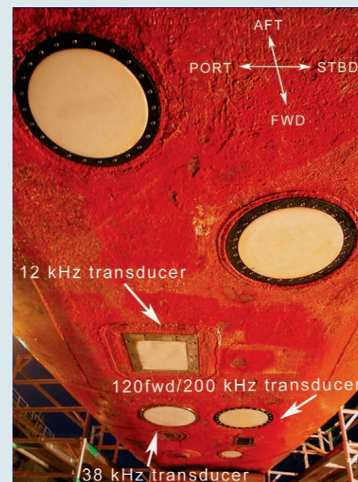
The echosounders on the RSV Aurora Australis are mounted in the hull and point downwards. During HIPPIES, data was collected from the sounders labelled ‘12’, ‘38’ and ‘120fwd/200’.
