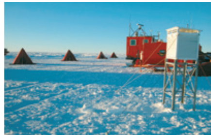
Stephenson screen houses thermometers used for daily weather observations
