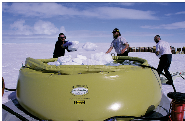
The 'flubber' used as a surface supply of water for the hot water drill in the Amery Ice Shelf glaciology program.
