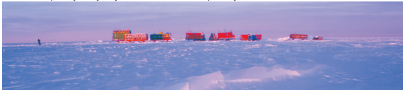
Traverse vehicles – fuel sledges, living van, generator van and tractors – at rest for the night while en route to Mt Cresswell.
