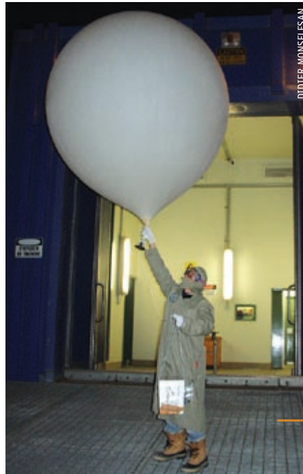
Bureau of Meteorology observer Annette Schlub launches an ozonesonde balloon at Davis.
