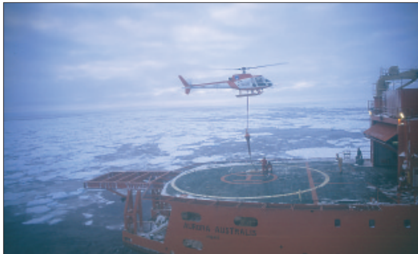
(left) MetOcean buoy is deployed by helicopter.
