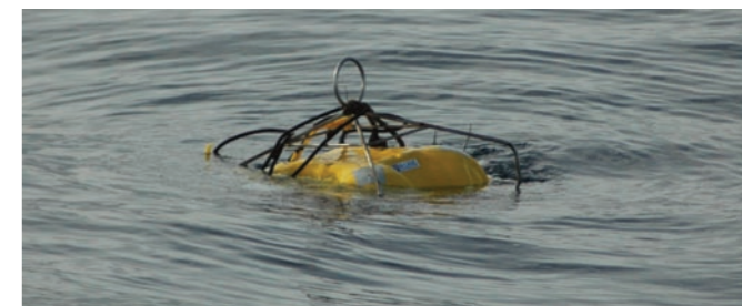
Technology that enables the remote collection of scientific data, such as this autonomous acoustic recording package used to capture underwater sounds, will play an increasingly important role in future marine research.
