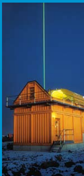
Above: Remote measurement of the atmosphere with a high intensity laser. From the returning light we get the temperature and amount of aerosols at all levels between 20-60 km altitude. Photo: Malcolm Lambert
