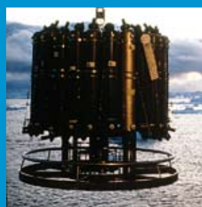
Above: Instruments are lowered thousands of metres into the depths of the ocean to measure the ocean salinity, temperature and oxygen content, and to collect water samples. These observations build a picture of the composition, structure and circulation of the deep ocean, and of its role in the climate system. Photo: Mark Underwood
