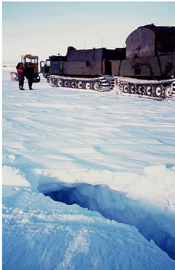
Figure 18: A crevasse discovered during attempts to prepare a skiway at Mirny for the Twin Otter
