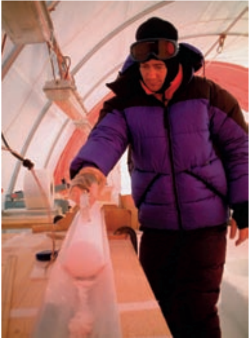
Ice core chemist, Mark Curran, measures the ECM of the ice core to determine its age.
