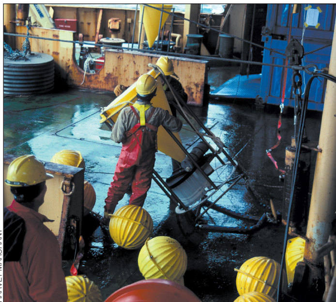
Instruments called sediment traps are used to determine what and how much of the biological production in surface waters is transported to the deep ocean. Here a sediment trap, one of an array of three, is about to be deployed. The array is anchored to the seafloor with the concrete weight (top left) and held upright in the water with floats - the yellow spheres (bottom right). This array will be recovered after collecting sedimenting material on a monthly basis for a year.
