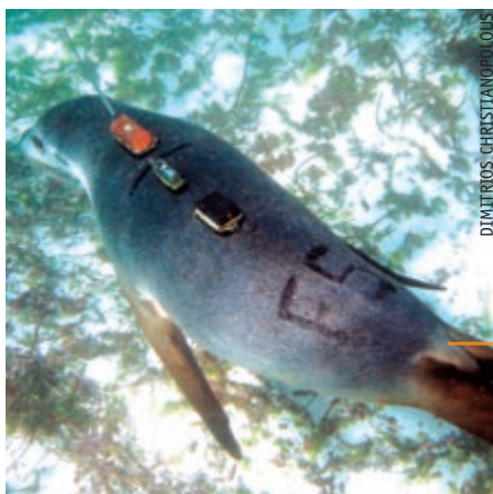
A juvenile Australian sea lion fitted with a satellite tracking instrument, time-depth recorder and VHF tag. Data from these instruments will help scientists understand more about the animals' foraging behaviour and range.
