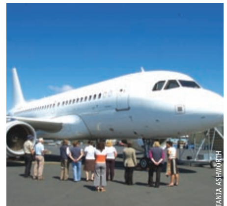
The A319, seen here being inspected by AAD staff in Hobart, is shorter than the A320 (used by Jetstar), and its under-floor cargo space has been commandeered to carry fuel, rather than baggage.
