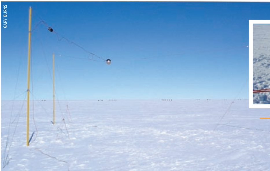
The Air-Earth Current Meter deployed at Vostok. This instrument measures the miniscule current (about 6 picoamps per square metre) flowing from the ionosphere to the ice through the suspended split-sphere. A picoamp is 10^{-12} of an ampere – approximately 160 000 000 000 times smaller than the current through a 60 watt light bulb.
